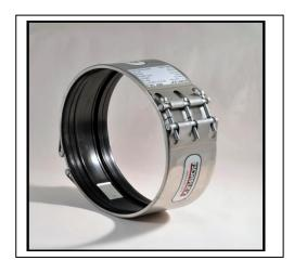
As we informed as above, again ground movement or the pipes where they will be joinined with angle on, the coupling can be made installation with 5° until DN300, 3° for between DN300-1000, 2° for above DN1000. Grip type coupling until DN600mm can be easily used for this kind of connections with angleANGLE IN **ELONGATION AND SHORTENING POSITIONS** WHILE CLAMP IS CONNECTED TO TWO PIPES.
